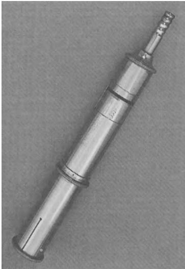
Fig. 1.1. Galton's whistle. The frequency of the tone emitted by blowing at the end of the whistle is dependent on the length. Zwaardemaker employed a series of whistles of different lengths to test patients with old age deafness.
