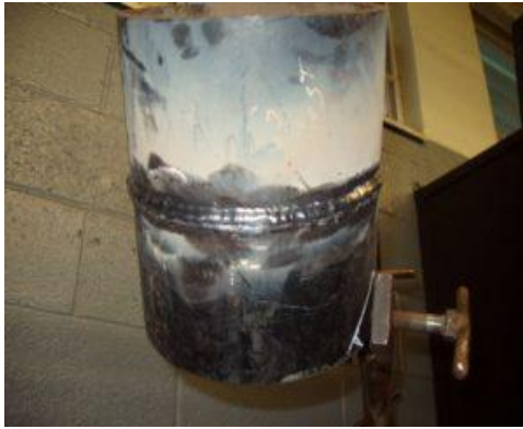
Bottom half of the pipe with 2 rows of cleaned stringer beads.
