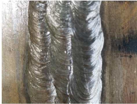
Figure 4.2 Fusion on weld face and toes.
