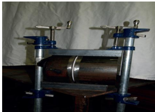
Figure 1.16 Channel Iron Used for alignment.
