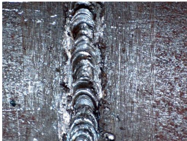
Figure 4.1 Fusion on the root side-both beveled pipe edges are melted.
