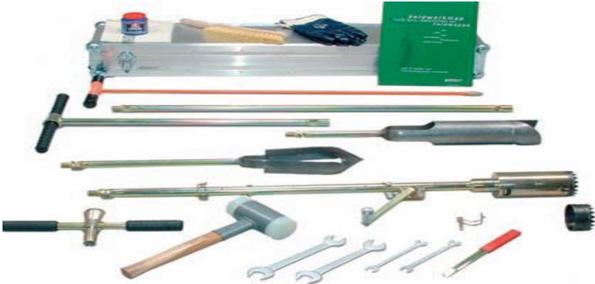
Fig: 1.2. Root Sampling Auger Kit; Standard Auger Handle; Beating Head Handle; Conical Screw Thread, 39.3 in (100 cm) Long Extension; Root Drilling Crown; Shock Absorbing Hammer; Utility probe, Spanner (wrench) 20x22mm; Field Data Registration set; Work Gloves pair; Maintenance Kit; Spatula bent.
