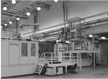
4.34 In-line compounding and injection moulding (Husky 5 ).
