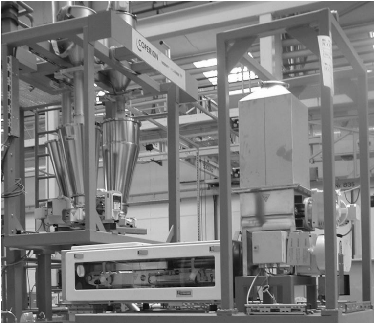
4.10 Weight belt feeder with a pre-feeding system (photo by Coperion Werner & Pfleiderer 2 ).
