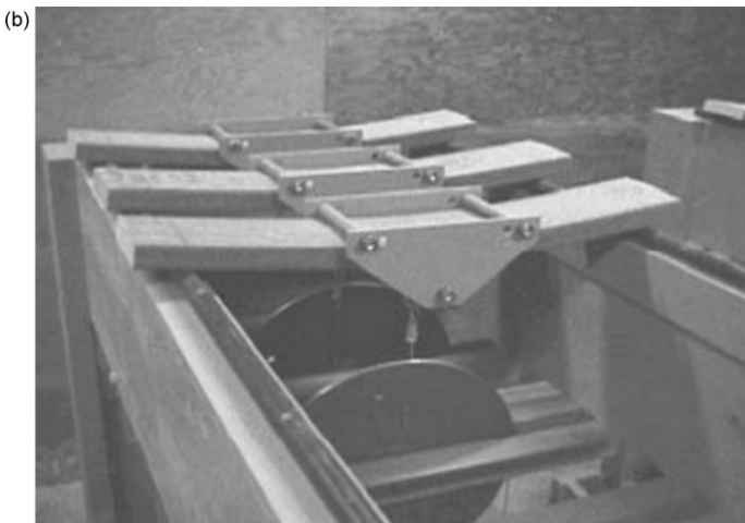
8.6 Life-size testing geometries: (a) three- and (b) four-point bending. From Tichy (2007).
