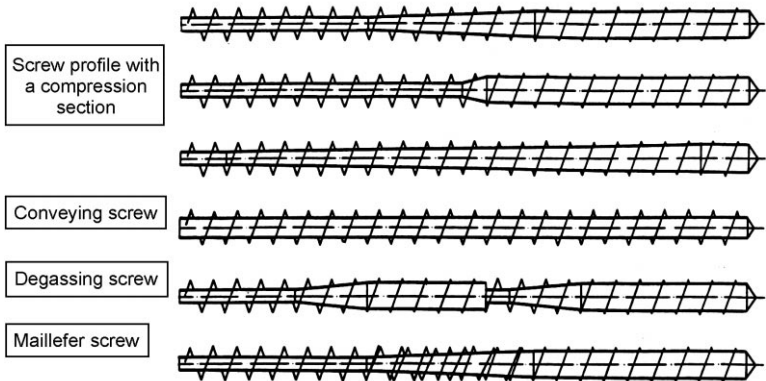
4.14 Basic screw designs of a single-screw extruder (Saemann 3 ).
