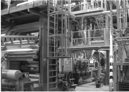
4.36 In-line compounding and sheet extrusion on a roll stack (Isokon 6 ).
