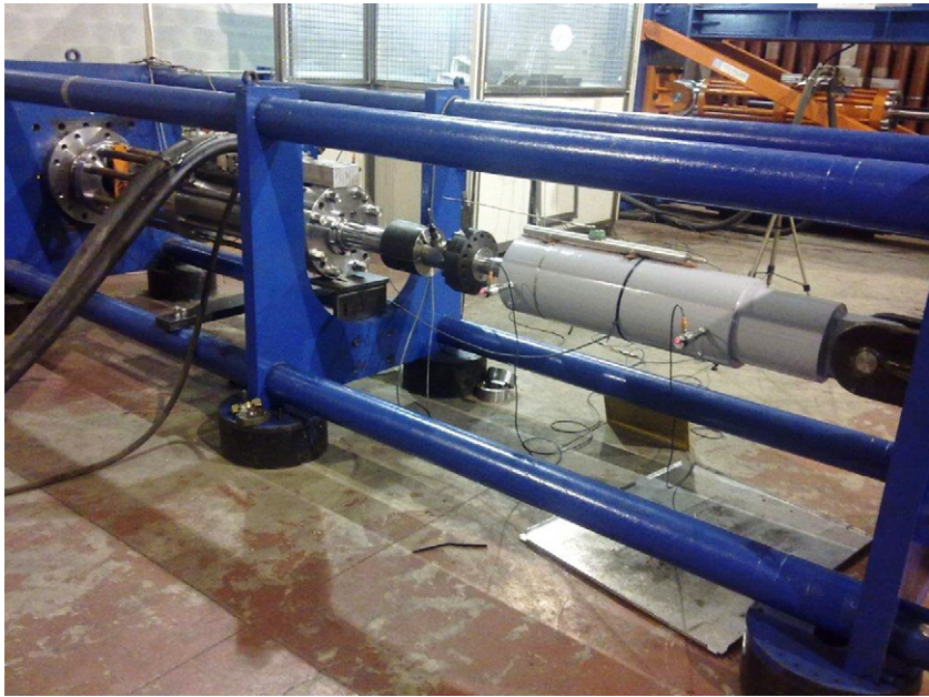
Figure 15.1 Viscous fluid damper installed on a damper testing machine.
