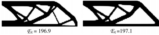
Figure 11.9 Two different topologies with nearly identical strain energy values.
