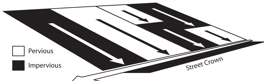
Figure 5.2 Diagram illustrating the layout of an urban element and all six possible contributing areas.
