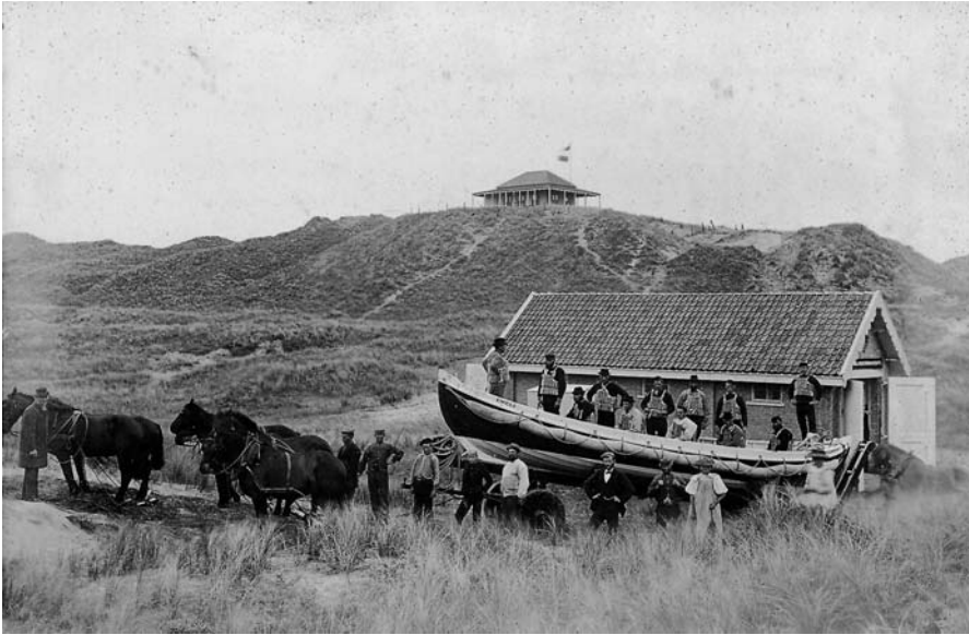
Fig. 1.2. A highly manoeuvrable clinker double ender with overhanging spoon bow and stern post. These boats were located in the village behind the dunes. When put into action, the local horses were gathered to bring the boat into the water. The seven rescuers then had to row to the endangered ship. This often took several hours
