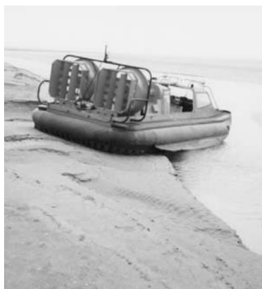
■ Fig. 5.22. The inshore rescue hovercraft makes the transition from water to land
