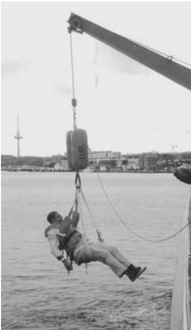
■ Fig. 5.12. Rescue lifting system (RLS Type B). This device with a “stopperblock” is used for rescue operations from high-sided ships
