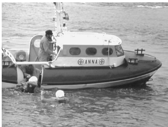
Fig. 5.7. The rescue boats and the daughter boats of the rescue vessels of the German Maritime Rescue Service (Deutsche Gesellschaft zur Rettung Schiffbrüchiger) have side doors close to the level of the water surface to pull in persons nearly horizontally
