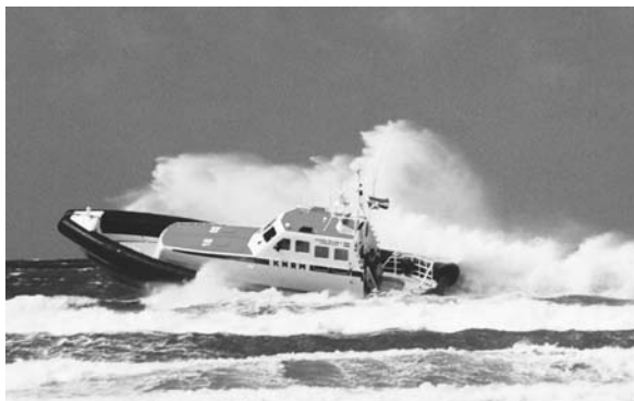
■ Fig. 5.18. The 62-foot RIB of the Arie Visser class
