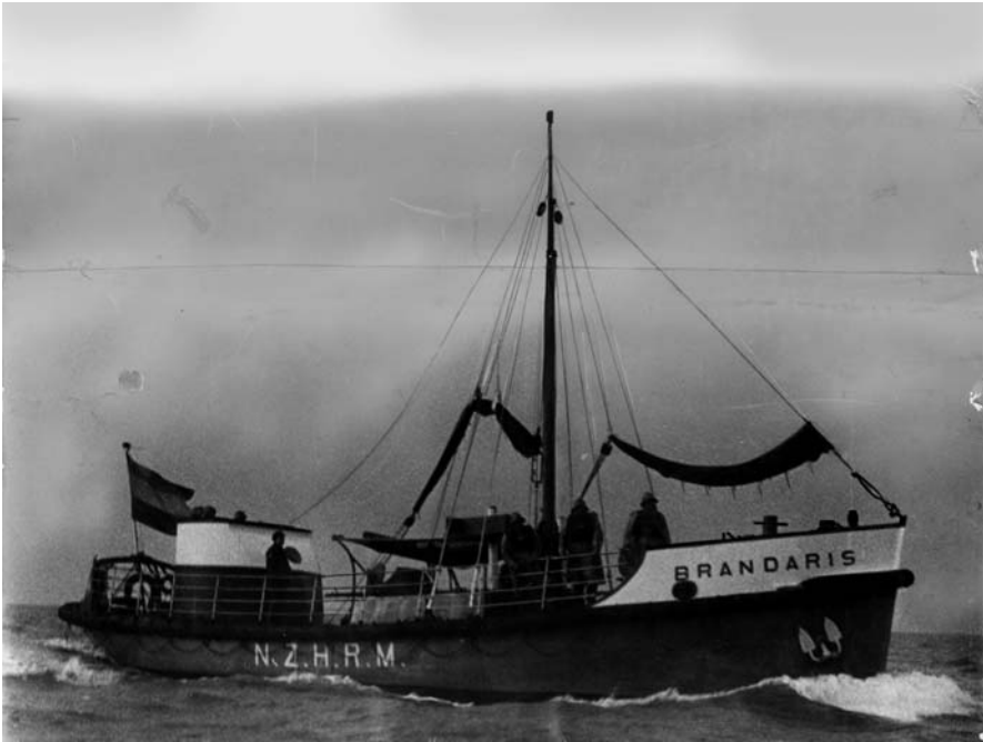
■ Fig. 1.4. In the beginning of the twentieth century, the first models of motorised rescue boats had a watertight engine room, a heavy bronze crew shelter aft and a jumping net
