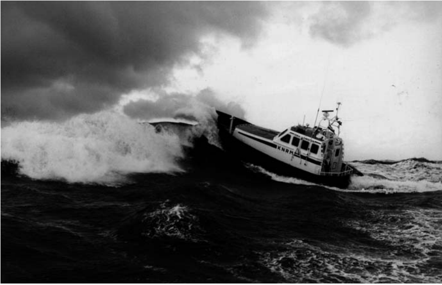
■ Fig. 1.5. Fast and manoeuvrable rigid inflatable boats (RIBs) were developed in the last decades of the twentieth century. Each RIB can float on its hulls without the tubes, but they can also float on the tubes alone
