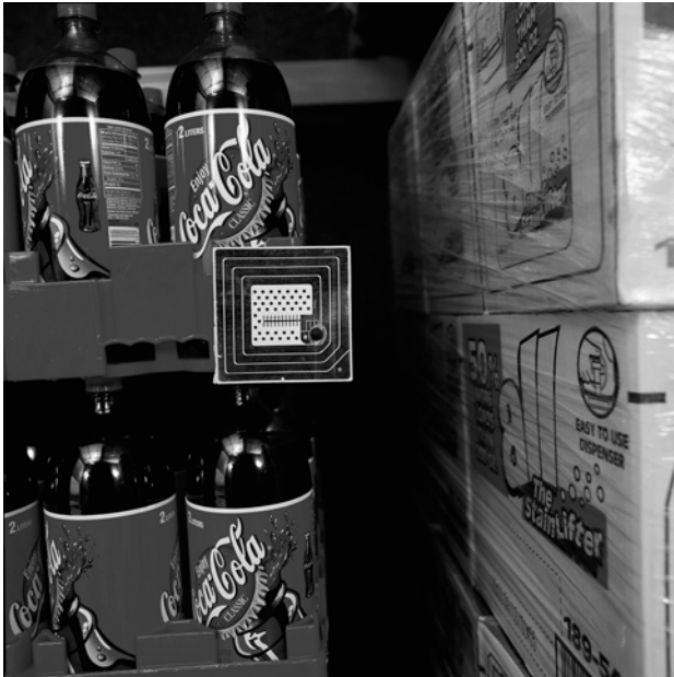
Figure 2-1 – A Passive RFID Tag
