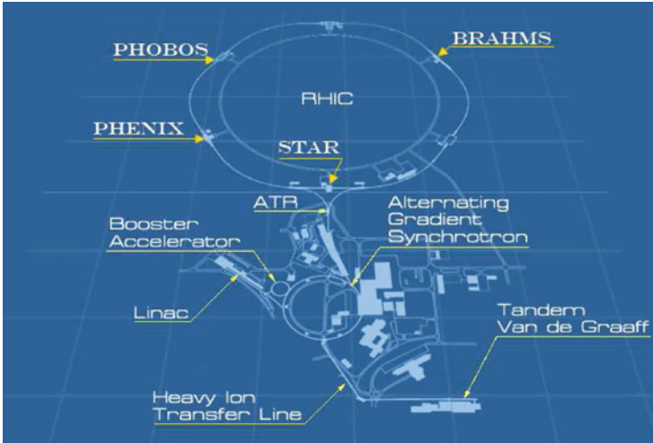
Fig. 2.1 The schematic plot of the Relativistic Heavy Ion Collider (RHIC) facility located at Brookhaven National Laboratory (BNL) (Diagram taken from [3])
