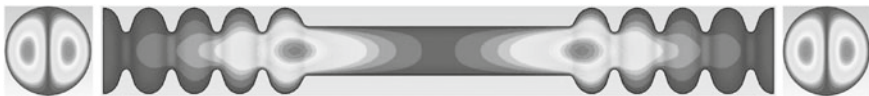
Fig. 2.13 The electric field distribution of one dipole beam-pipe mode (frequency: 4.1481 GHz, R/Q : 1.544 \Omega/\text{cm}^2 ). Electric (EE) boundary conditions were used in the simulation
