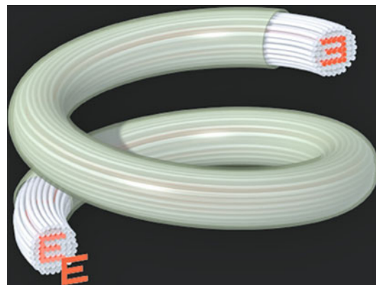
Fig. 2.25 Rastered imaging through an image-conducting fiber optic cable. Each fiber produces a point of light. The diameter of the fibers limits the resolution. This principle is applied in the endoscope
