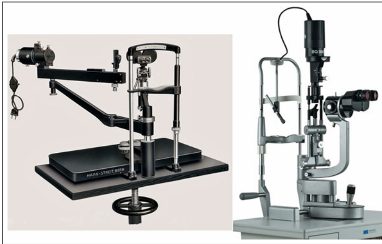
Fig. 4.14 Left: Goldmann slit lamp (1933). One recognizes the stereomicroscope and the projector for the slit light. Right: modern model. (Courtesy of Haag-Streit AG, Switzerland)
