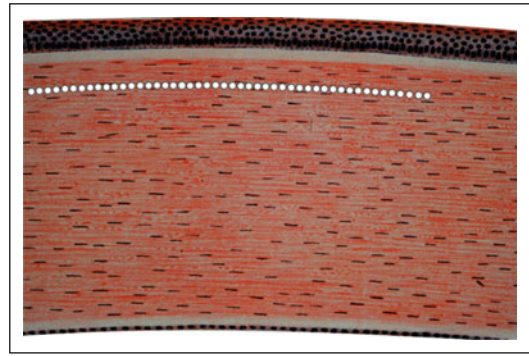
Fig. 7.25 Schematic drawing of the impacts of femtosecond laser pulses. Optical breakdowns create numerous tiny bubbles with diameters of a few \mu\text{m} . They form a two-dimensional carpet of adjacent vesicles. In reality, the bubbles are smaller than drawn here
