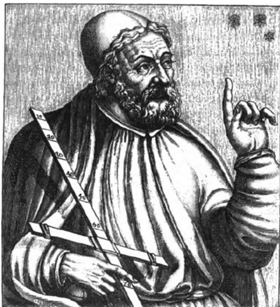
Fig. 1.1 An imagined depiction of Claudius Ptolemy holding a cross staff (some historians have traced the origins of the cross staff to the Chaldeans in 400 BC) used to measure the separation between stars from the book Great Astronomers by Sir Robert Stawell Ball, published by the J.B. Lippincott Company in 1895
