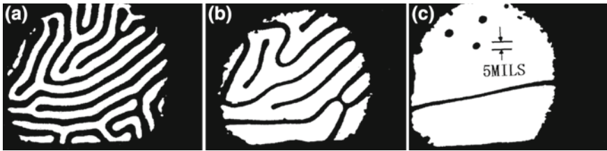
Fig. 7.11 Formation of magnetic bubbles (Kerr effect patterns). H = 0 (a); 1.6 \times 10^3 A/m (b); 2.2 \times 10^3 A/m (c) [5]
