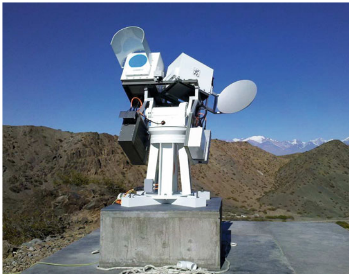
Fig. 8 The solar patrol polarimeters completed for installation at El Leoncito Observatory. The 90 GHz 22 cm aperture at the left side and the 45 GHz 44 cm at the right side produce a 1^\circ beam for full sun regular observations
