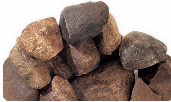
Fieldstone is stone gathered from fields, dry riverbeds, and hillsides. It is used in wall construction.
