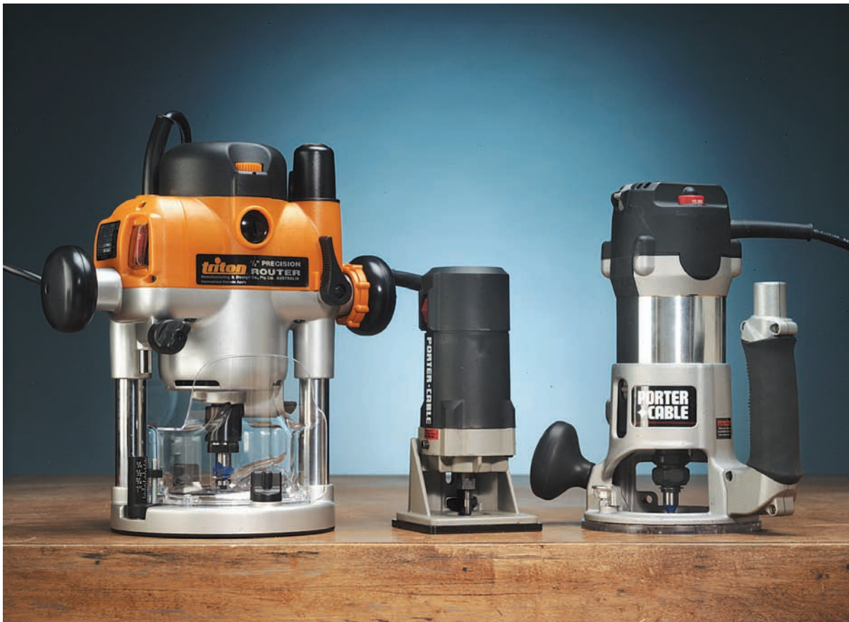
The plunge router (left) and fixed base router (right) are the two main types of routers for general workshop use. A trim router (center) is smaller and used primarily for trimming plastic laminate.
