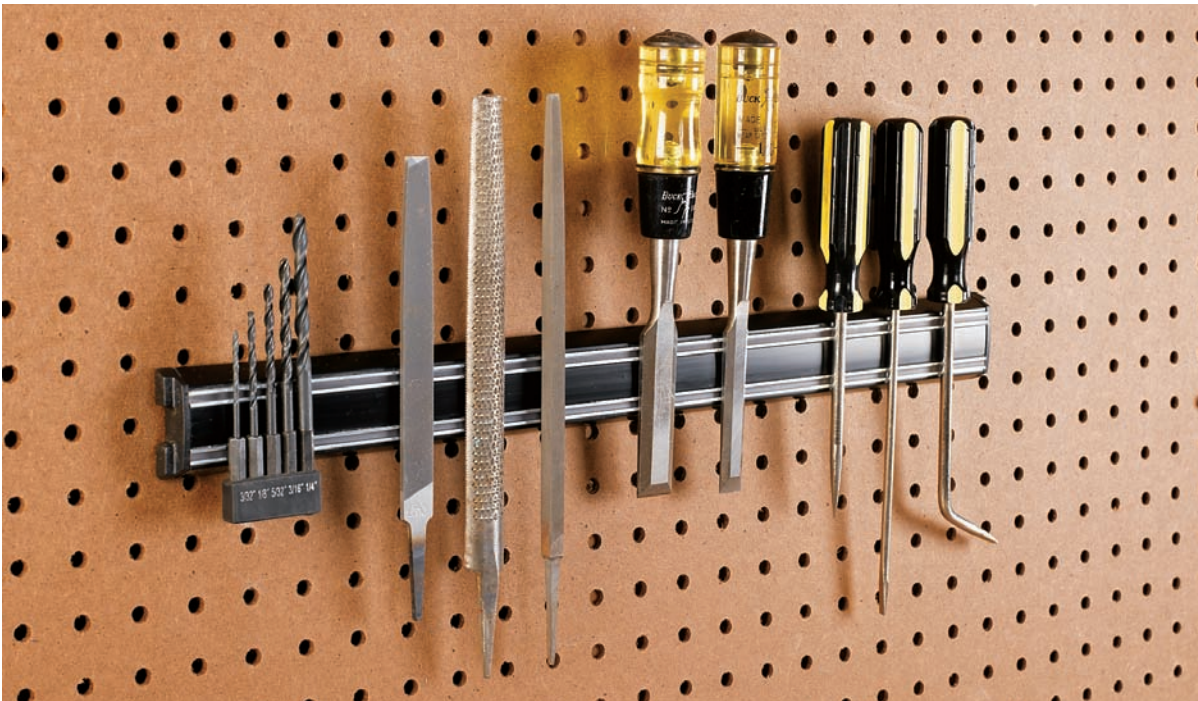
Magnetic bar strips , typically used for holding knives in the kitchen, are just as handy for storing chisels, files, awls, and other metal tools in the workshop.
