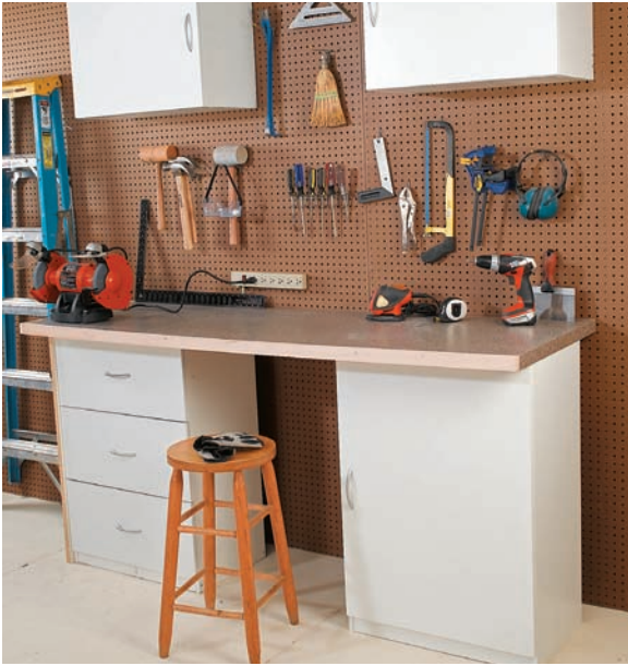
A utility shop. This compact shop area was made with inexpensive utility cabinets and a plywood work top.
