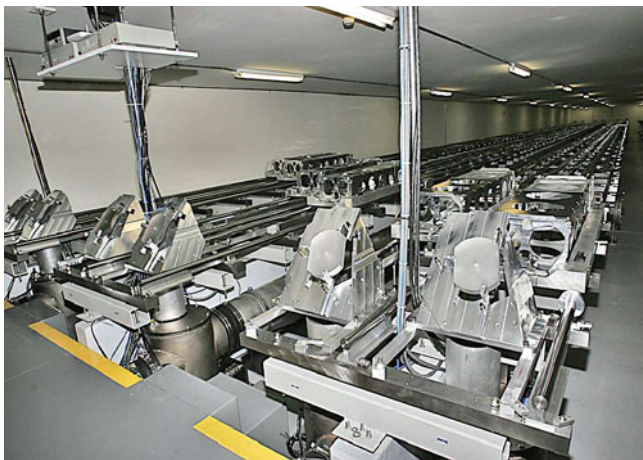
Fig. 7.9 The Optical PathLength Equalizers (OPLE) are placed on rails 50 m long, giving up to 100 m of delay controlled to an RMS of 10 nm (courtesy: S. Golden)
