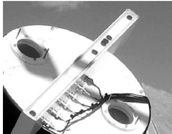
Fig. 4.6 SHABAR uses six photo-diodes attached to a single aluminum I-Beam providing a maximum baseline of 46.87 cm, which was mounted over the telescope with the Solar Differential Image Motion Monitor (SDIMM). The position of the individual sensors in the array are placed at different locations, which act as a miniature telescopes with 7^\circ field-of-view (FOV). They are separated by 15 non-redundant baselines. The cross-correlations of the measurements over several possible detector separations can be inverted to estimate r_0 as a function of height. This instrument was procured from National Solar Observatory (NSO), USA and installed at the Indian Astronomical Observatory, Hanle (courtesy: S. P. Bagare)
