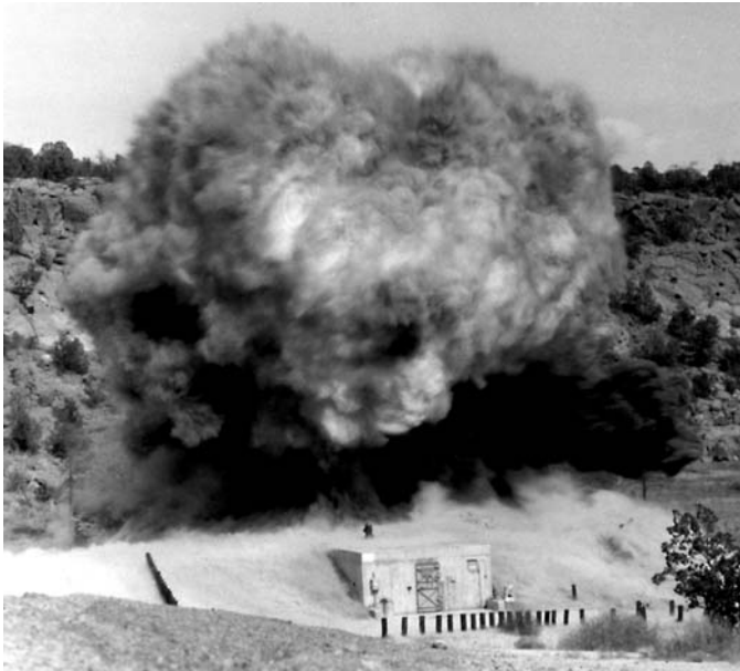
Fig. 1.1. Photograph of a large piece of condensed-phase high explosive detonating at a firing bunker at Los Alamos National Laboratory. To give an idea of the scale of this picture, the door on the bunker at the bottom of the picture is about 1 m wide.
