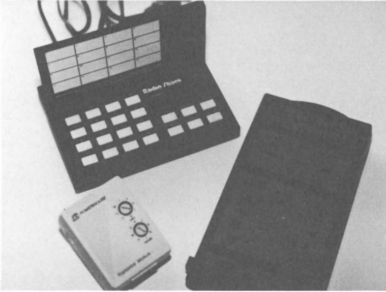
Figure 6.12 X10 controller and module, TASH infra-red controller.
