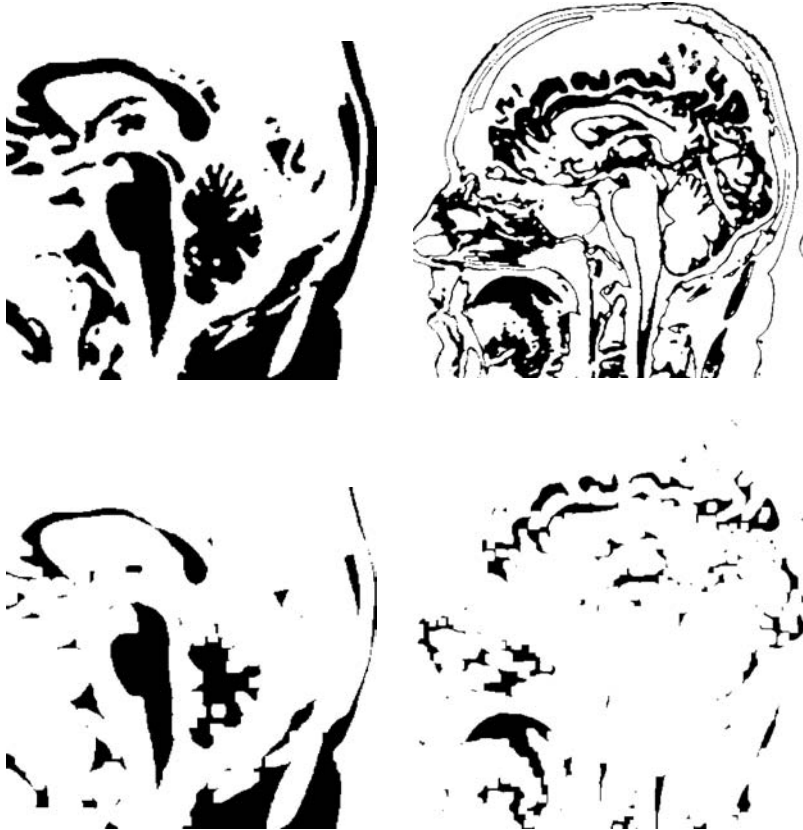
Figure 13.24 (Above) Example of two binary images and (below) their erosion by the centered 7 \times 7 mask.
