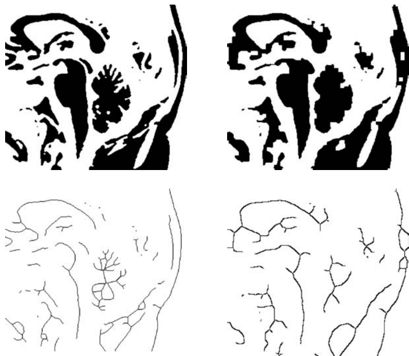
Figure 13.29 Below: Skeletons of a binary image and its closing (above). Note the influence of border complexity on the skeletons.
