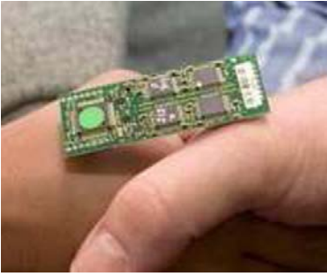
Figure 8. A closeup view of the electronic readout board of ALICE dimuon spectrometer showing four MANAS chips
