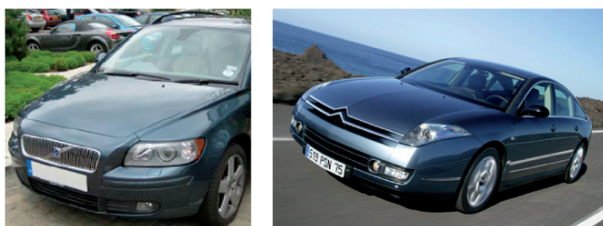
Fig. 10.23 Moving the bonnet leading edge rearward: Volvo S40 and Citroën C6, adapted from [65].
