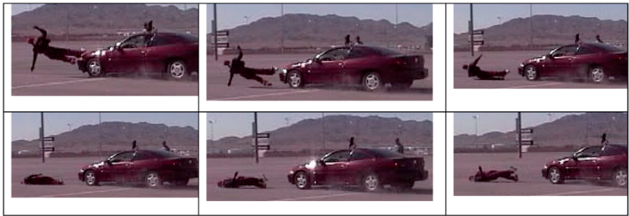
Fig. 9.1 Post head impact kinematics in a staged test showing slide, roll and bounce in ground contact, adapted from [8].
