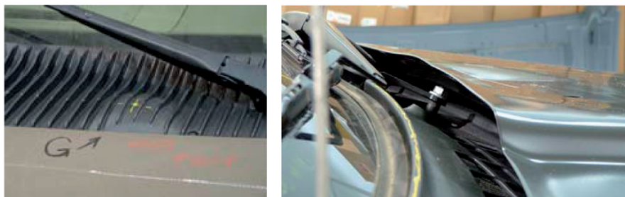
Fig. 10.29 Exposed cowl and covered cowl, adapted from [105].
