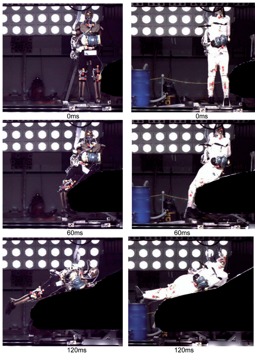
Fig. 8.1 Comparison Polar II pedestrian dummy (left) and cadaver (right) kinematics a 40 km/h lateral impact with a recent small passenger car, adapted from [10].
