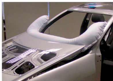
Fig. 10.31 Bonnet lift by airbag to protect head from A-pillar and lower windscreen frame contact, adapted from [111, 112].
