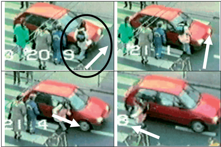
Fig. 3.3 Real-world low velocity pedestrian sideswipe collision in Helsinki: arrows show the direction the woman is facing [21].
