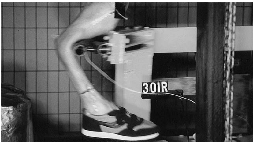
Fig. 1. Cadaver test simulating a pedestrian impact.
