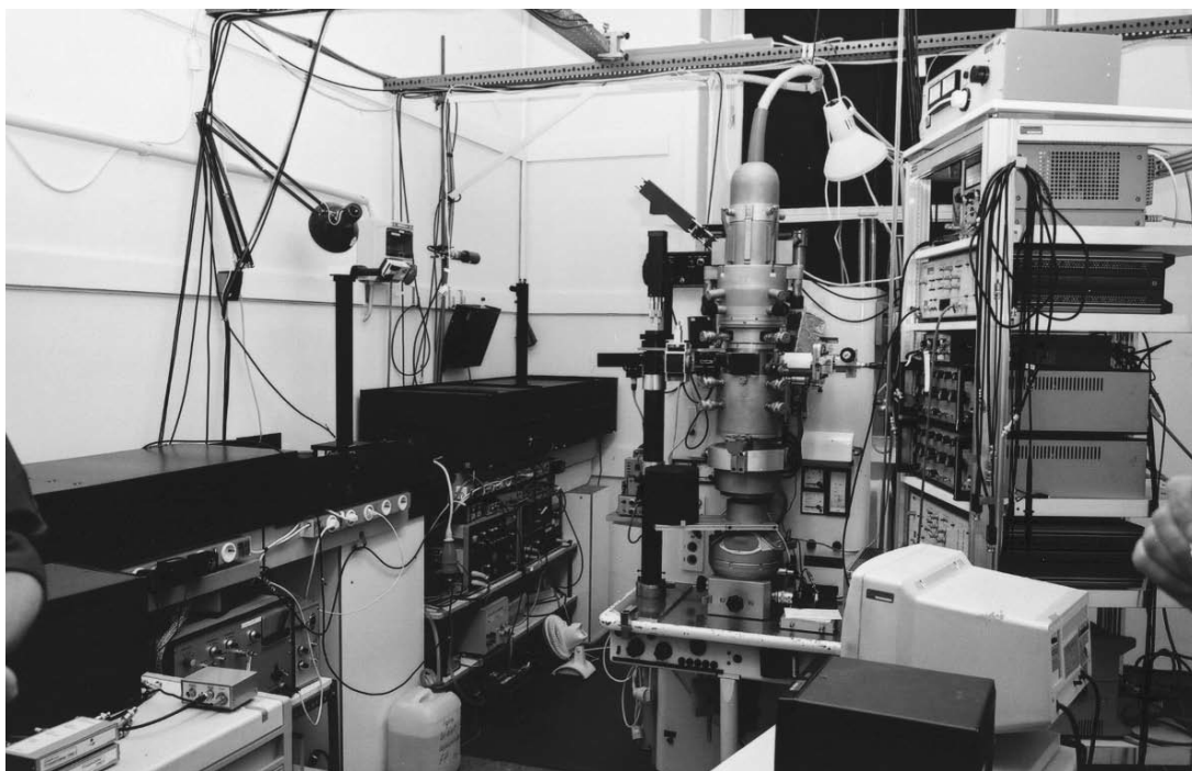
Figure 5–2. The DTEM at TU Berlin. Cathode and sample drive lasers are at left. (See color plate.)
