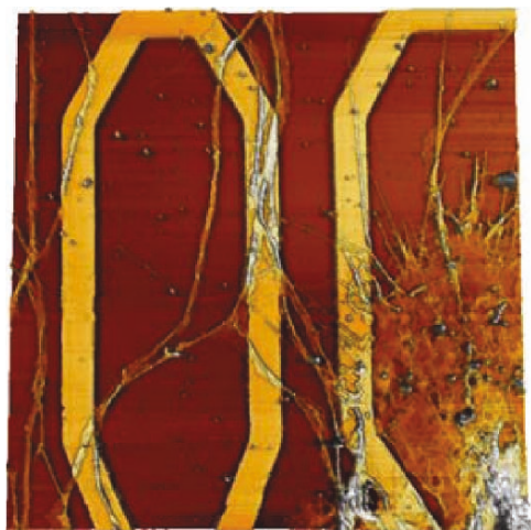
Figure 16-3. Neuronal cell, cultured on an electronic chip. The chip is designed such as to pick up an action potential of the cell. The image demonstrates proper tracing of the cell surface. In a future application, an appropriately designed stylus might be used as an additional electrode to excite or record an action potential at any location of the cell body or a process of the neuronal cell.
