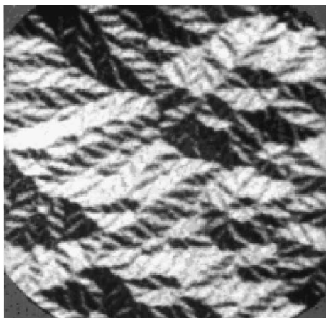
Figure 8–37. SPLEEM image of the closure domains on a Co(0001) surface. Electron energy 2 eV. 279
