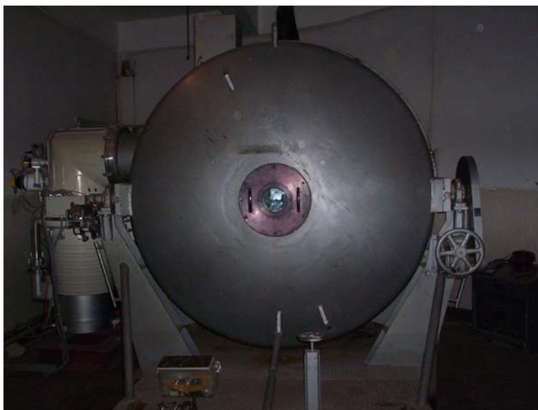
Fig. 4 Upgraded Kottamia 74'' mirror aluminizing plant
