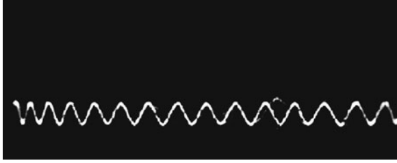
Fig. 10.17 Self-excited vertical oscillations of a particle in the sheath of a dc discharge, which is moving horizontally from left to right. This photo has an exposure time of 0.88 s. (Reproduced with permission from [269]. ©1999 by the American Physical Society)
