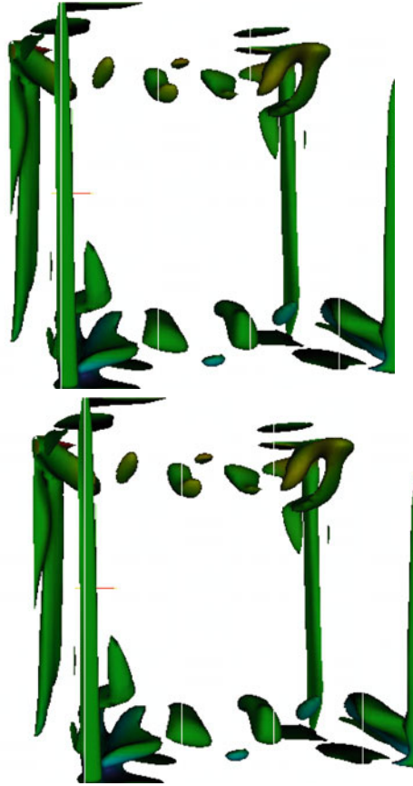
Fig. 4. Instantaneous x component of vorticity obtained at Ra = 3.5 \times 10^6 . The front is the cold wall at x = 1 . On the left, the 2D centro-symmetry in (x,z) is imposed while on the right the full 3D centro-symmetry has been forced.
