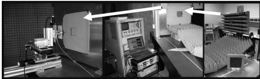
Fig. 11.50. Experimental test setup for measuring PIM, NIM, and GRIN spherical lenses. The plane wave is generated at the right, travels through the aperture in the center panel, and is detected by the receiver on the left. The experiment is controlled by a computer running Labview shown in the center panel
