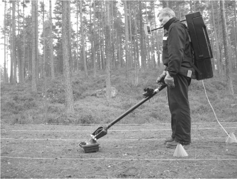
Figure 3.1. The HUMUS GPR system and operator. The computer screen displays depth view of the waveforms, detection alerts, and possible mine classification results.
