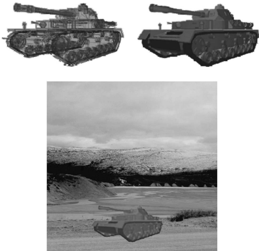
Figure 8.1. A set of synthetic test images: a wireframe model of the target (top left), a realistic solid model of the target (top right), and a realistic scene with the target (bottom).
