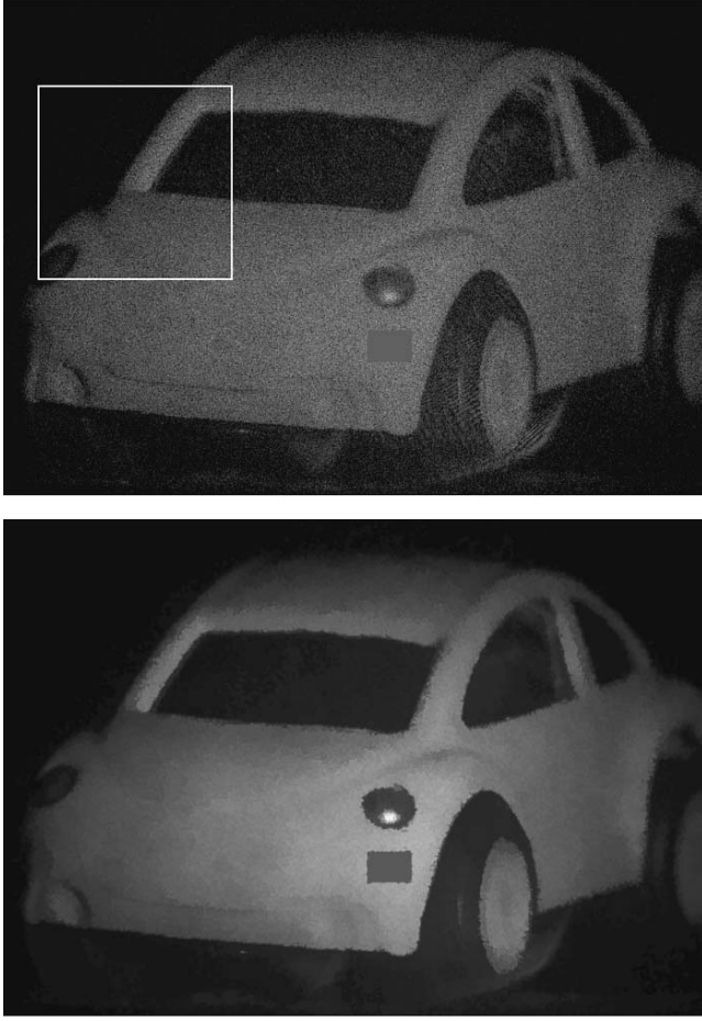
Figure 13.7. (top) Reference image of a toy car reconstructed from an experimental digital hologram 1123 \times 1585 with 1-order speckle (or 1 look). Drawn with modification of gray-levels for visualization. White box correspond to the part used in Fig. 13.3 (bottom) Result with 5 pixels base triangle, \mu = 20.0 and \beta = 0.3 . (27s, 222437 nodes, PIII-1.1GHz).
