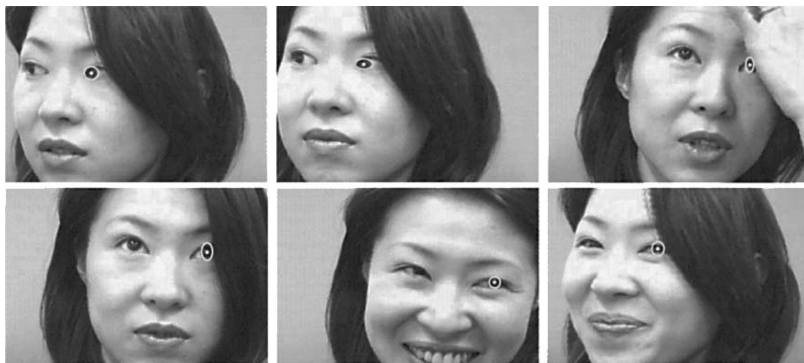
Figure 9.20. Tracking results of the left eye using the PF-iris based tracking algorithm described in Figure 9.19. Note the occlusion of the tracked eye by the subject's hand and hair.
