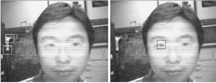
Figure 9.10. Illustration of some steps of the dark-bright pupil-based approach: initial list of potential eye candidates (a), and final list of detected eyes (b). Note that the two false eye candidates are rejected using a SVM classifier.
