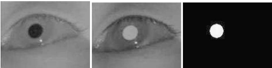
Figure 9.4. Examples of a dark and bright pupil images and their corresponding pixel-to-pixel enhanced subtraction image.
