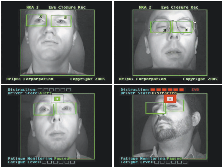
Figure 9.21. Snapshots of two applications of eye tracking: (1) fatigue assessment : the eye state is classified as open (top left) or closed (top right); and (2) distraction assessment : as the head pose is frontal (bottom left) or non-frontal (bottom right) for a while, the driver is recognized as non-distracted (bottom left) or distracted (bottom right). Both eyes were detected and tracked in real-time. Some human factor algorithms being used to measure distraction from the head pose classification results can be found in [18, 19, 24] (see color insert).
