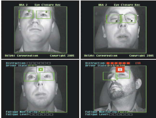
Figure 9.21. Snapshots of two applications of eye tracking: (1) fatigue assessment : the eye state is classified as open (top left) or closed (top right); and (2) distraction assessment : as the head pose is frontal (bottom left) or non-frontal (bottom right) for a while, the driver is recognized as non-distracted (bottom left) or distracted (bottom right). Both eyes were detected and tracked in real-time. Some human factor algorithms being used to measure distraction from the head pose classification results can be found in [18, 19, 24].
