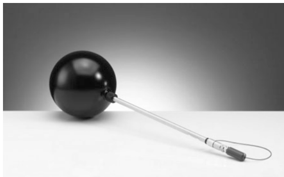
Fig. 2.35 Absolute dosimeter to measure kerma in the air, air-equivalent ionization chamber PTW
