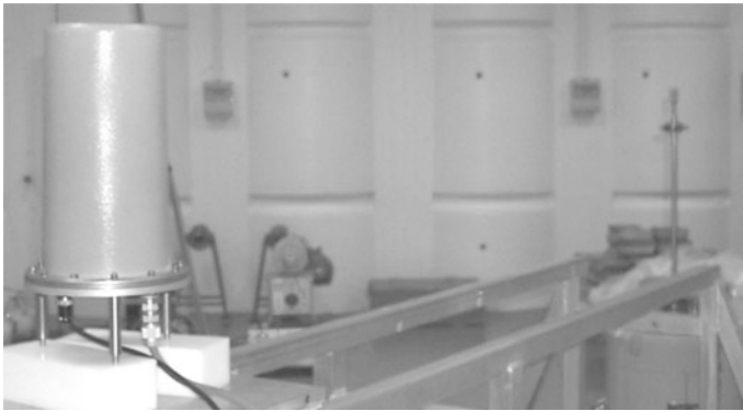
Fig. 3.42 Calibration of the radiation protection device on the calibration bench, here \gamma ionizing chamber in a secondary laboratory
