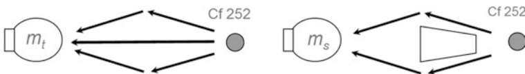
Fig. 3.44 Raw and scattering measurements for neutron device calibration using the “shadow cone” technique
