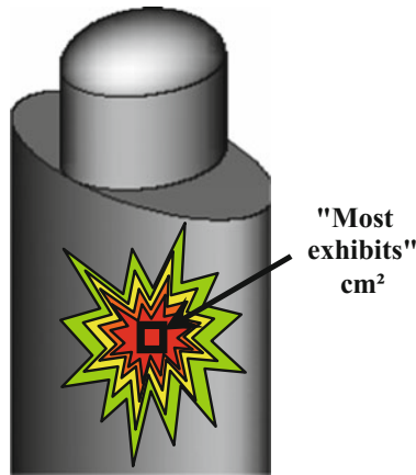
Fig. 3.4 Illustration of the region of greatest exposure for the calculation of the equivalent dose to the organ H_{skin} in the context of extremities exposure
