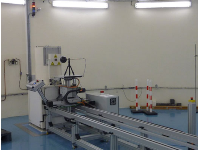
Fig. 3.41 Secondary laboratory bench during a connecting process for the measurement of air kerma with PTW chamber and a point-source
