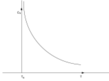
Figure 1.9. Constant volume specific heat near the liquid gas critical point.
