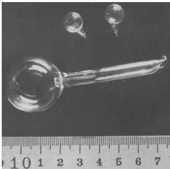
Fig. 25 The mercury in the irradiated gold foil is melted with an induction heater, driven to gold catchers, and finally to the resonance cell or lamp
