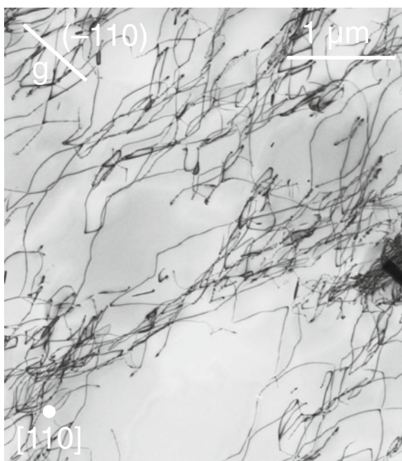
Fig. 9.42. Dislocation microstructure of \text{MoSi}_2 deformed along [110] at 380^\circ\text{C} from the same deformation experiment as Fig. 2.6. Foil plane parallel to the (110) cross section plane. From [15]. Copyright Wiley-VCH (2005)
