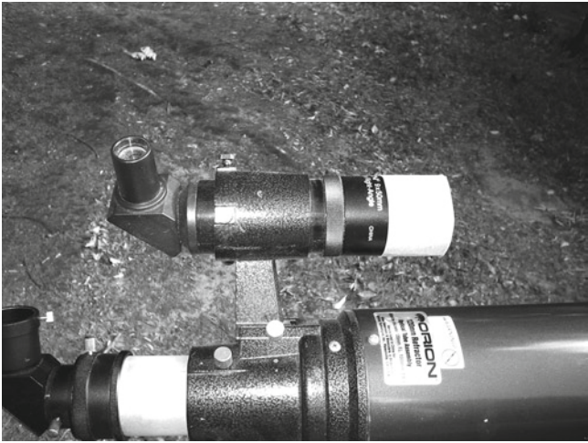
Fig. 4.22. A homemade dew-shield on a finder (credit: Richard W. Schmude, Jr.).
