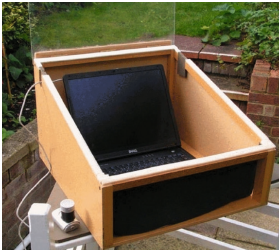
Fig. 9.1. Computer 'dry box' (Credit: Chris Hooker).
