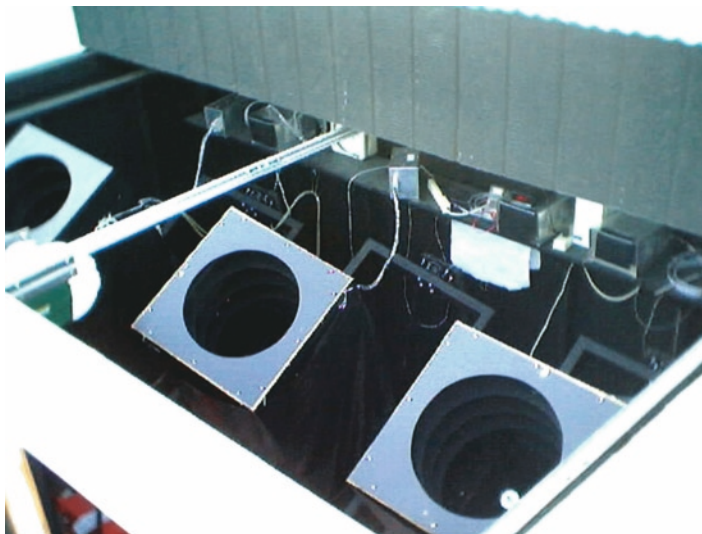
Fig. 11.11. Moving Object and Transient Search System (MOTESS) telescopes (Credit: Roy Tucker).
