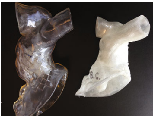
Fig. 10.2 Using the data from CT or MRI scans, 3D printed outflows are created. Using different printers and materials allows for either more rapid prototyping, or printing in different materials. The different materials allow for translucent printing on the left , and printing can be done in different materials of different compliance
