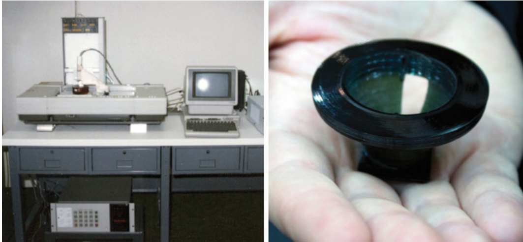
Fig. 1.4 First SLA machine build by Charles Hull in 1983, and the first object printed in that machine a cup that took months to finish. Courtesy of 3D System, Inc
