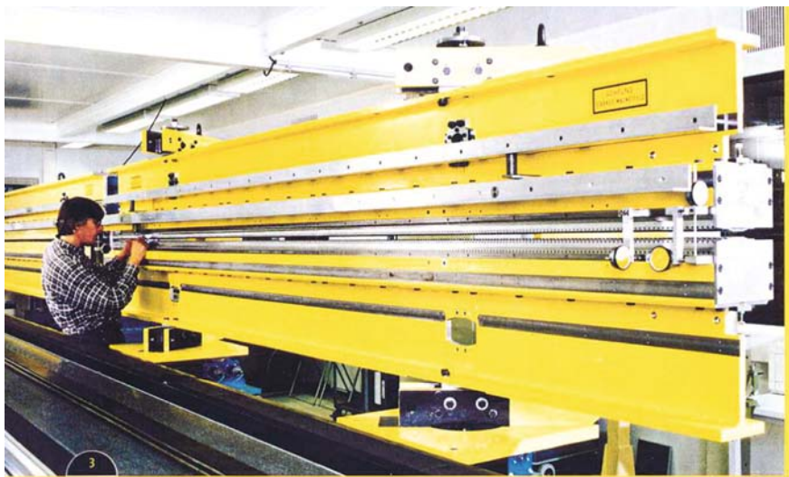
Fig. 8.12. Photo of a FLASH undulator magnet
