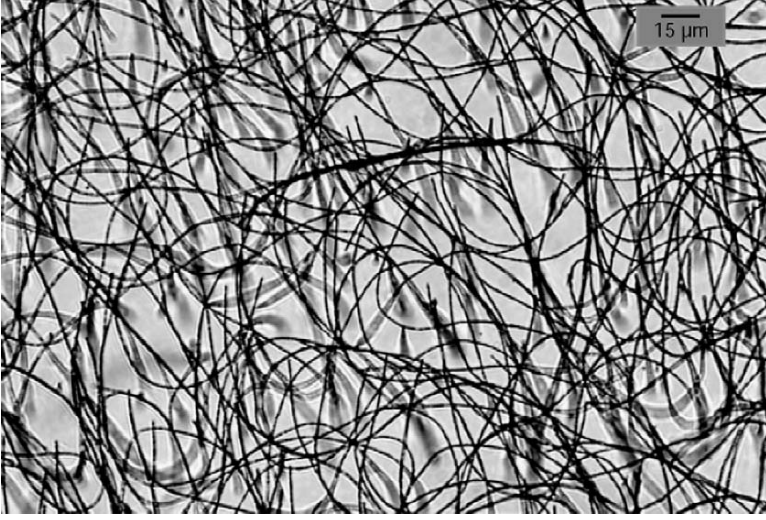
FIGURE 2.16. Long magnetic nanowires made by submitting a mixture of magnetic particles and PAA to a magnetic field. The chains are bent by gravity after field removal. (Reproduced with permission from [47].)
