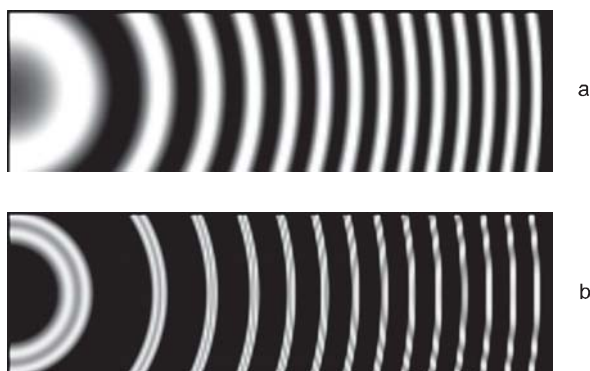
Figure 1.40. Spectra of the D -lines of sodium ( \lambda_1 = 589 nm, \lambda_2 = 589.6 nm) obtained with a FABRY-PEROT interferometer of h \approx 0.038 mm at R = 0.53 (a), and at R = 0.78 (b).
