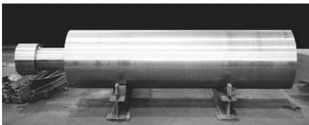
Figure 18. A 10-tons model steam turbine rotor made of designed steel.
