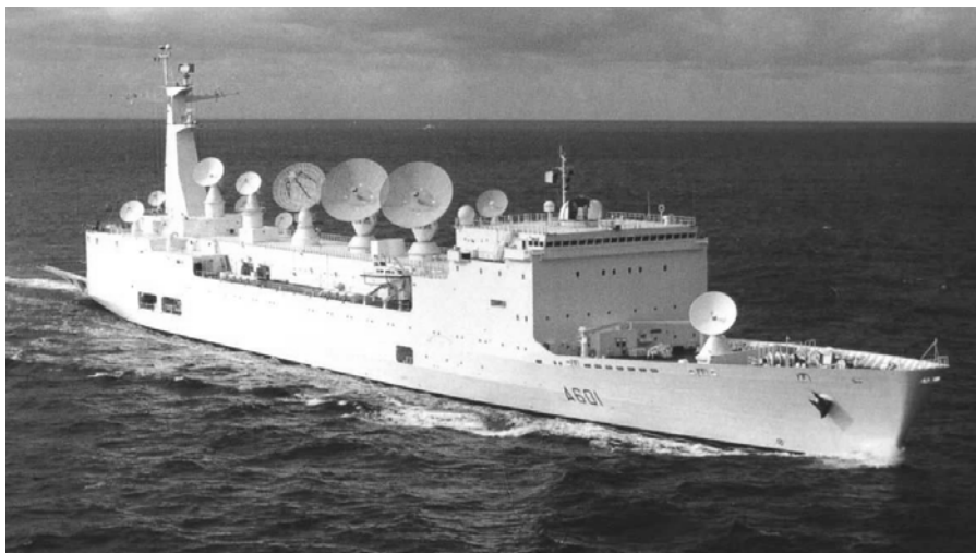
Fig. 2.31. The French tracking ship Monge with its Armor and Gascogne radars (source: DGA).
