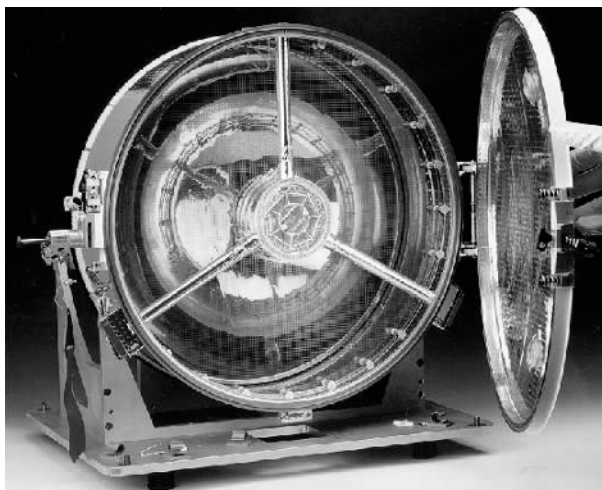
Fig. 2.36. The GORID impact plasma detector as used on the Ulysses, Galileo, and Ekspress-2 missions (sensor area: \sim 0.1 \text{ m}^2 ; source: ESA).
