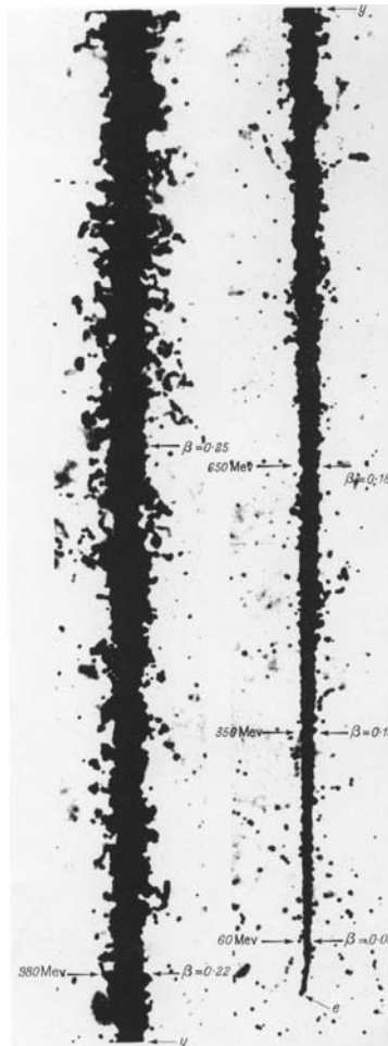
Fig. 2. — Track of a chromium nucleus of the primary cosmic rays, coming to rest in nuclear emulsion flown in a high-altitude balloon. Notice that the track tapers as the velocity of knock-on electrons decreases as the nucleus slows down, and it also begins to collect successively, first K -shell and then L -shell, etc. electrons.
