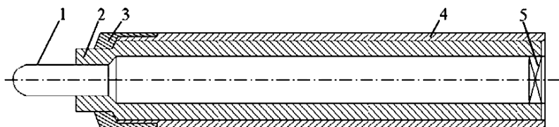
Fig. 3.1. Coaxial electrocontact sensor [3]: 1 – brass rod; 2 – electrical insulation; 3 – tip; 4 – sensor casing; 5 – mica washer
