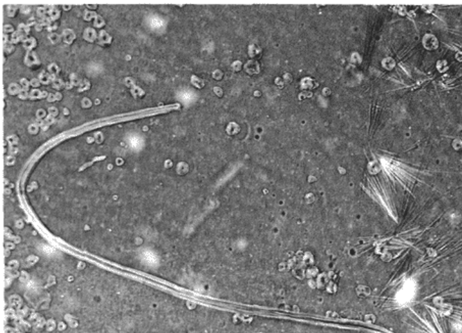
Fig. 3. Crystals of salts in a transparent adhesive tape preparation from a wall.
