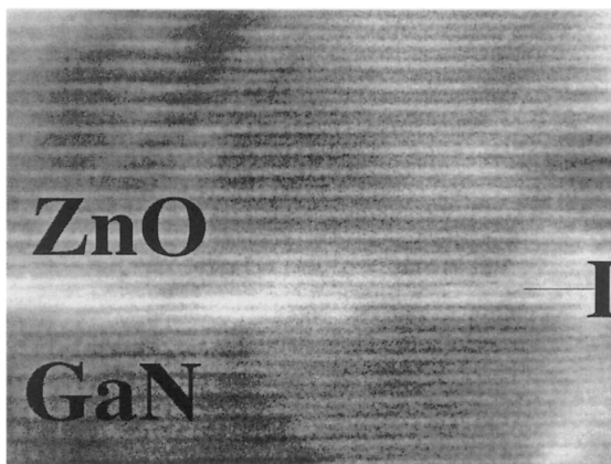
Figure 8: High Resolution Transmission Electron Microscopy image of ZnO on a GaN substrate. The interfacial region is marked with an "I".
