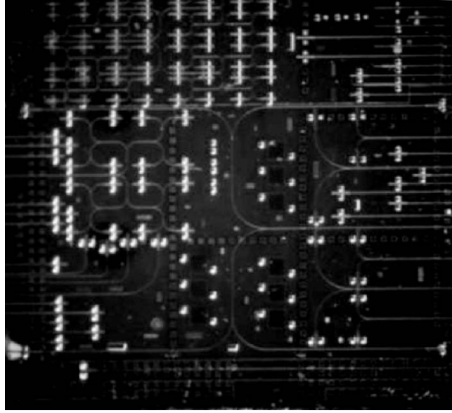
Fig. 11.6. Optical clocking chip. Used by permission from Intel Corporation as published in [13]
