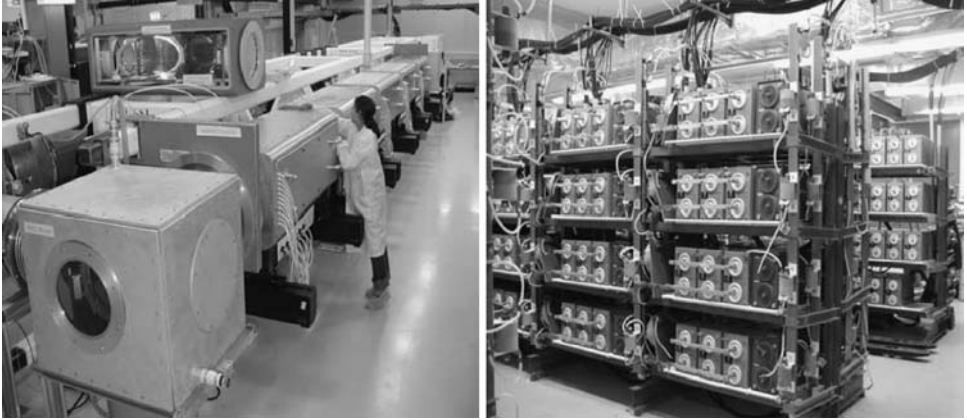
Figure 3. Double-pass section of the main amplifier ( left ) and capacitor bank ( right ).
