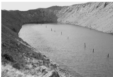
Figure 3. The Telkem2 crater produced on 12 November 1968 by the simultaneous explosion of three 240 t fission devices
