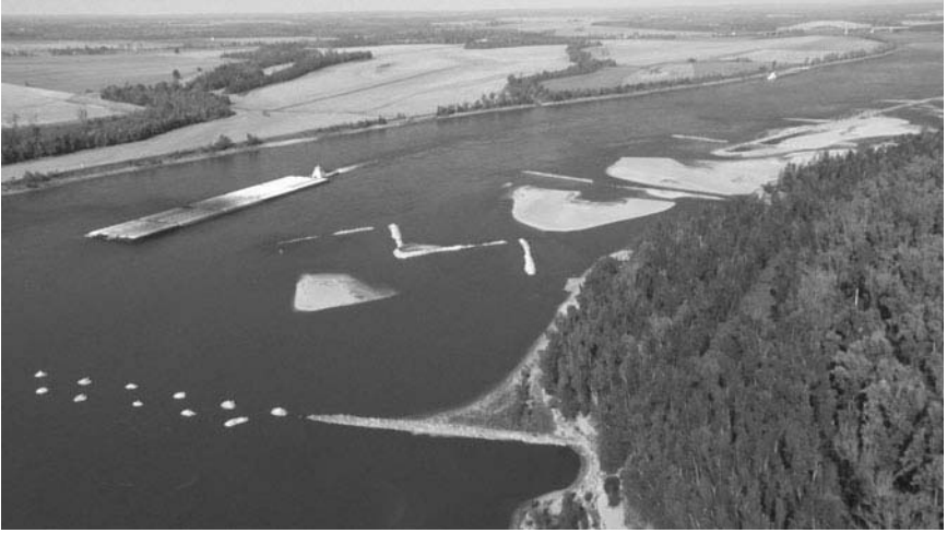
Fig. 1-1. Dikes and revetments on the Mississippi River Source: USACE St. Louis District
