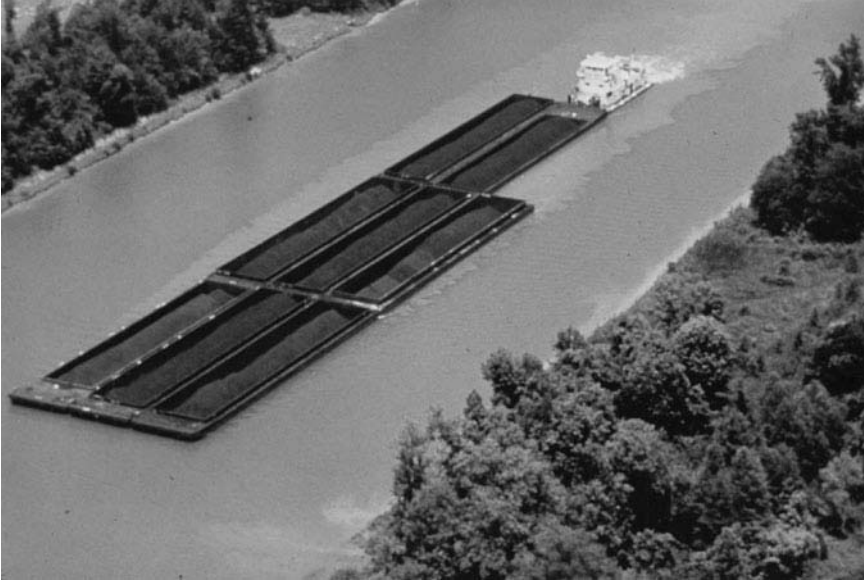
Fig. 2-1. Surface sediment plume from vessel passage Source: USACE Engineer Research and Development Center, Coastal and Hydraulics Laboratory
