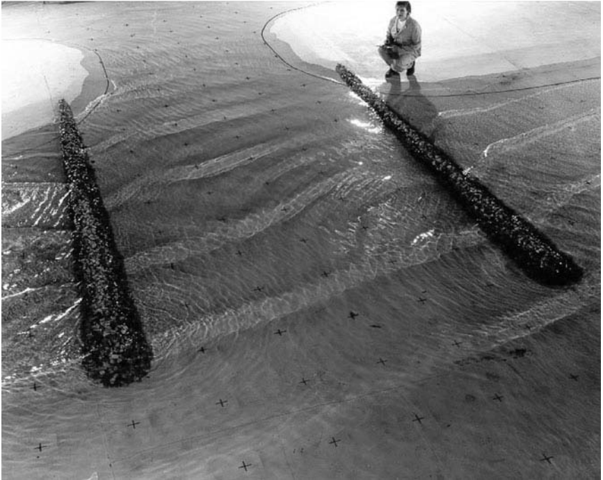
Fig. 11-1. Idealized model inlet in a physical model
