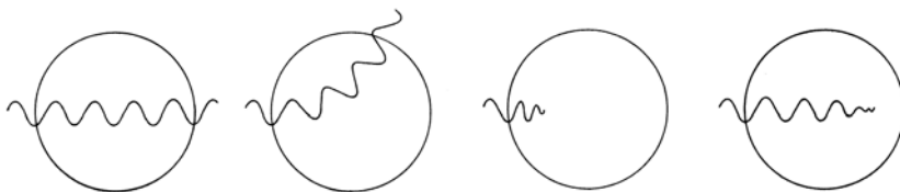
Fig. 12.1. Fate of excited wave: passing through, refraction and reflection, absorption near boundary, and absorption at center of plasma
